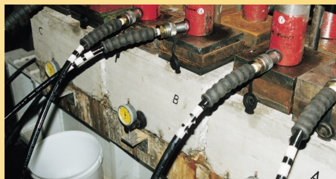
Testing for SikaSwell® expansion pressure development and pressure resistance according to STUVA
